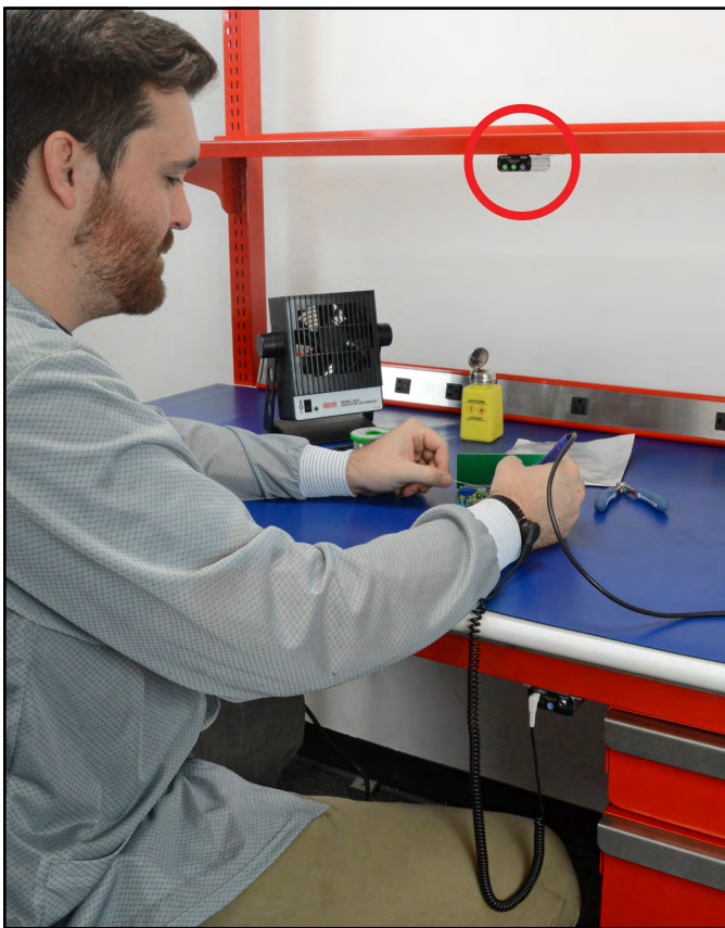
Figure 9. Using the 724 Plus Workstation Monitor when mounted underneath a surface
