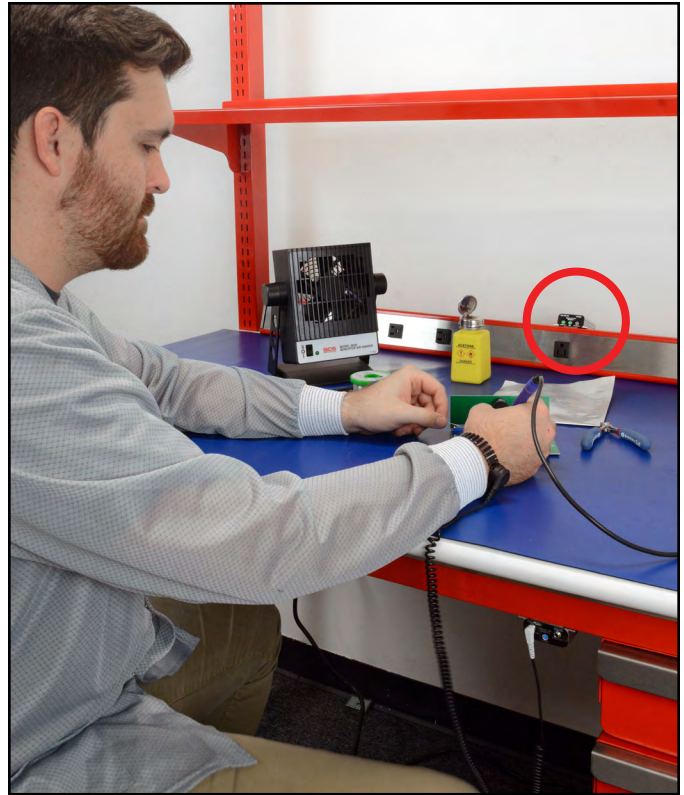
Figure 10. Using the 724 Plus Workstation Monitor when mounted on top of a surface
