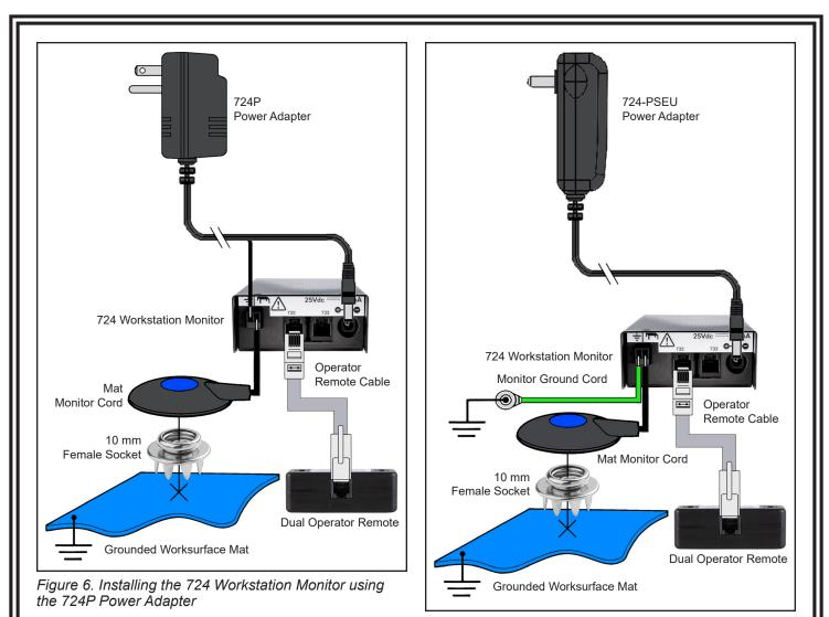
Figure 7. Installing the 724 Workstation Monitor using the 724-PSEU Power Adapter
